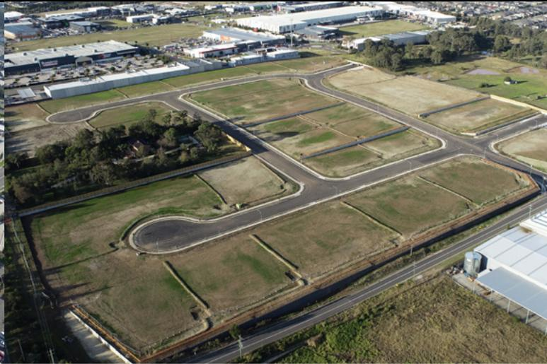
**Delivery of a commercial industrial development for Stockland including demolition, extensive remediation, bulk earthworks in rock, civil works inclusive of frontage upgrade to live road, installation and commissioning of services to lots.**
